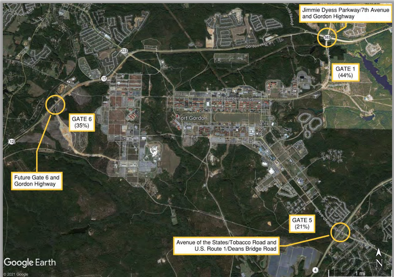
Figure 3.22: Future Access Gate Layout Used for the Existing and Future Model Analysis and Estimated Volume Share (%) by Gate. Map Source: Google Earth; Data Source: Stantec Consulting Services, 2021
