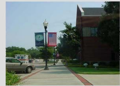
On-street parking, wide sidewalks and pedestrian-scale lighting are just a few of the features that can be incorporated into urban streetscapes.
